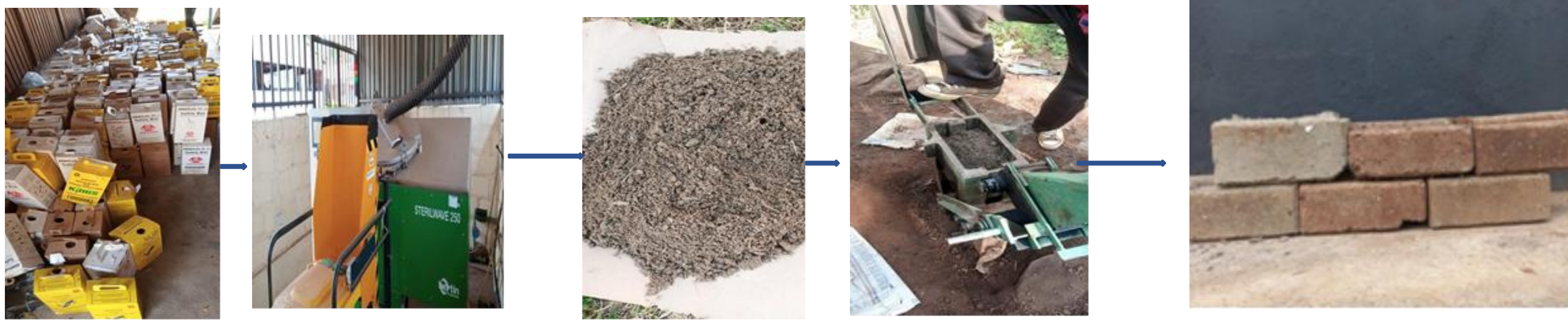
THE LINE PROCESS OF CONVERTING HEALTH CARE WASTE INTO BRICKS FOR REPURPOSED FOR USE AS SANITATION BLOCKS AND PAVING BRICKS.
